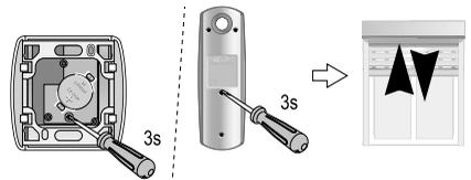
[5]. Check that pairing has worked by pressing the "Test" button.
