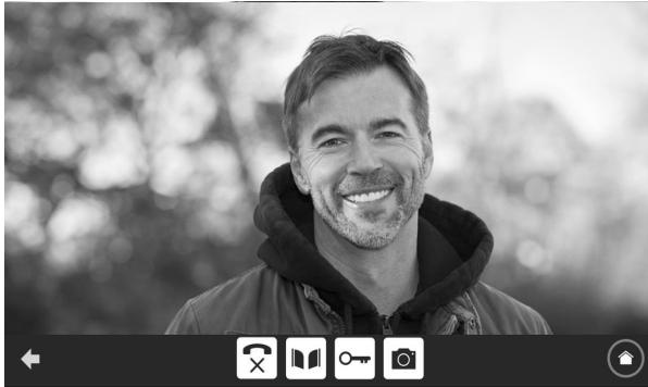
To take the call, press the "telephone off the hook" pictogram. The internal monitor's microphone and the door station's speaker are only activated once the call has been accepted.
